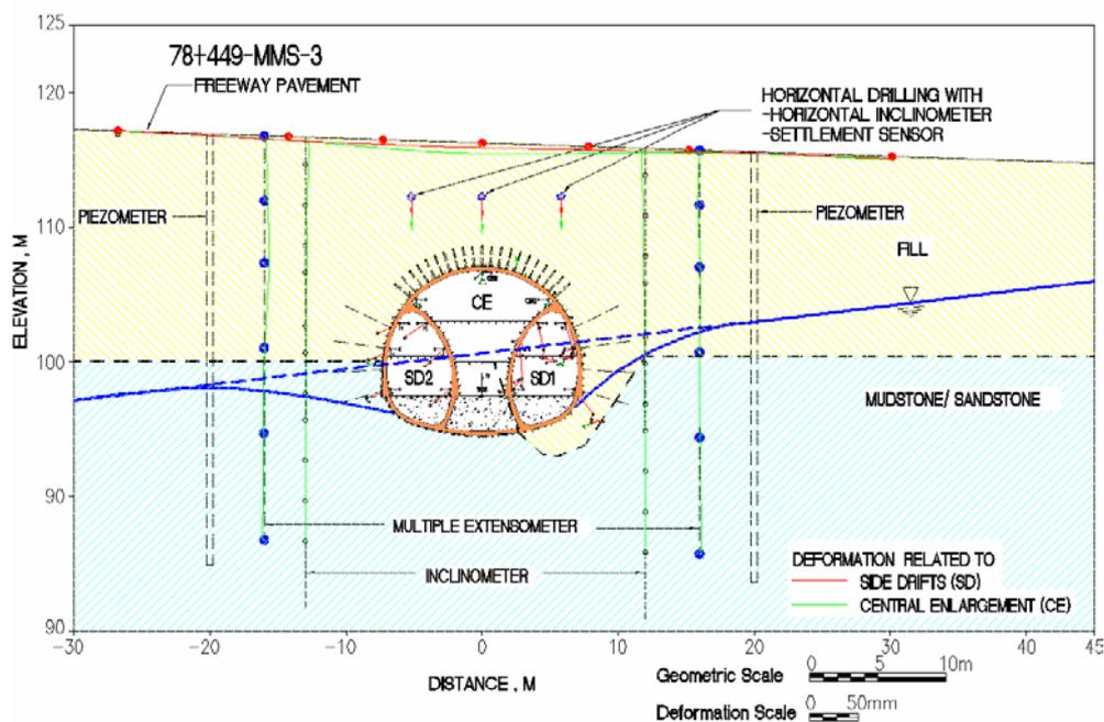
Figure 2: Main monitoring section 78+449 with monitoring results
