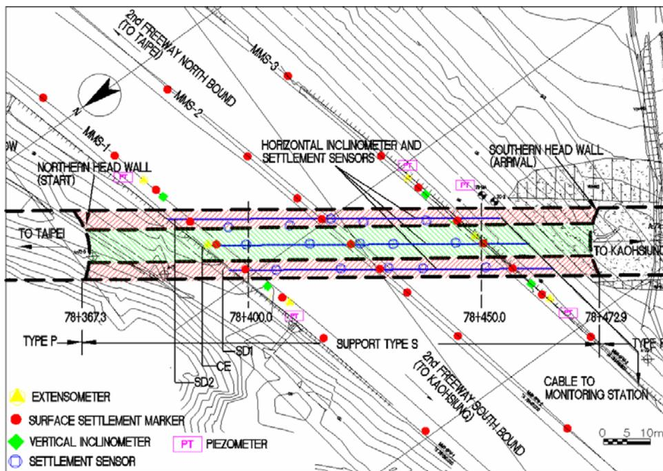
Figure 1: Layout of underpass site with monitoring arrangement
