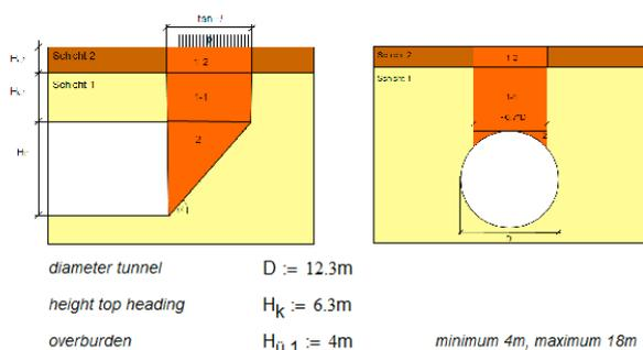
Figure 7: Geometry of failure wedge
