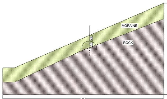
**Figure 5: Cross section 1, model geometry**
