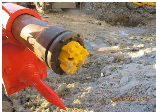
Figure 12: Drill head for steel pipes. Only the yellow drill part is retracted
