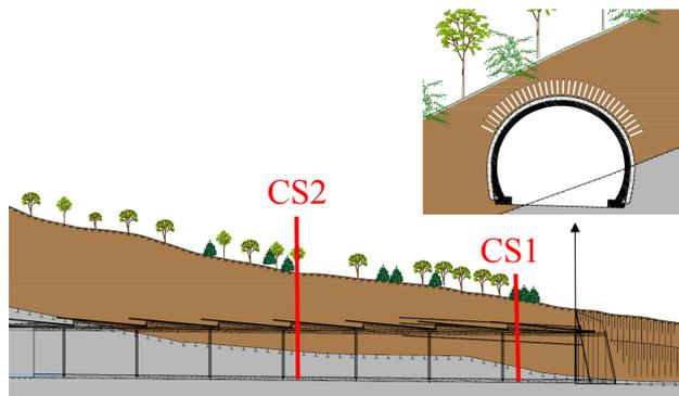
Figure 4: Longitudinal profile and cross section of the entrance point for the soil tunnel at Holven
