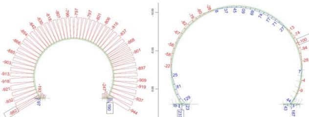
Figure 8: Critical load case, normal force left, bending moments right.
